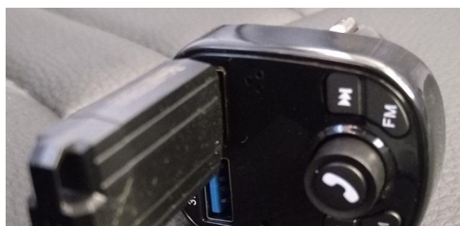
FM Transmitter and 16 Gig flash drive that plugs into the cigarette lighter socket
