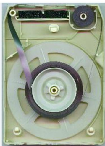
Inside of an 8 track tape, The tape is pulled off the inner part of the reel then fed back onto the outside, giving continuous playing
